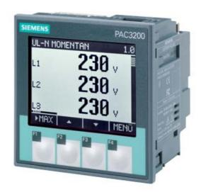
SENTRON PAC3200; LCD; 96X96MM POWER MONITORING DEVICE PANEL MOUNT TYPE FOR MEASUREMENT OF ELECTR. VALUES VAUX: 22-65VDC VIN: MAX. 500/289V; 45-65HZ AMPIN: X/1A OR X/5A AC COMPRESSION TYPE TERMINALS
